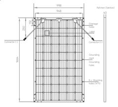
Module dimensions in the technical picture are expressed in mm with tolerance  $\pm 2$  mm ( $\pm 0.079$  ")
