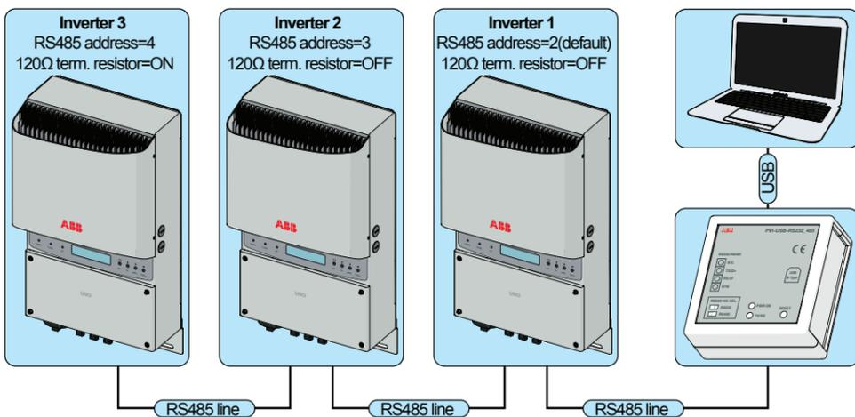
**Characteristics of application cables for the creation of the RS485 communication line**
